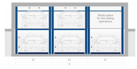
On the entrance level are sliding platforms with one empty space on the right (on the left: possible as an option). On the lower level the system is provided with lifting platforms. A lifting platform will be lifted to the empty space on the entrance level.
