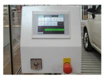
Operation by touch screen with key switch and emergency-stop. With brief operating instructions fastened on the wall and cabling to the power unit.
